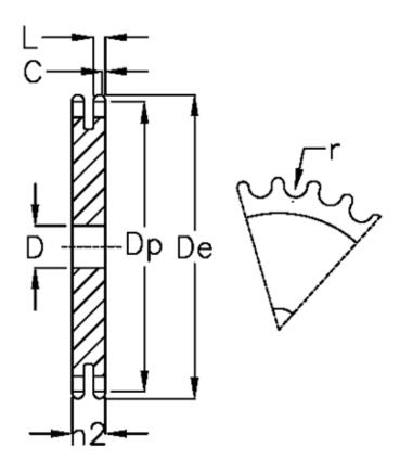
C = 2 D = 25 De = 367.5 Dp = 357.93 For chain size =  $3/4 \times 7/16$ For chain type = 12 B-2 h2 = 30.3 L = 10.8 Number of teeth = 59r = 12.07
